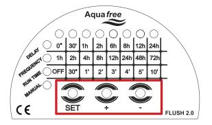
The flushing system is controlled with the three keys labelled "SET", "+" and "-" at the bottom of the operating panel.
